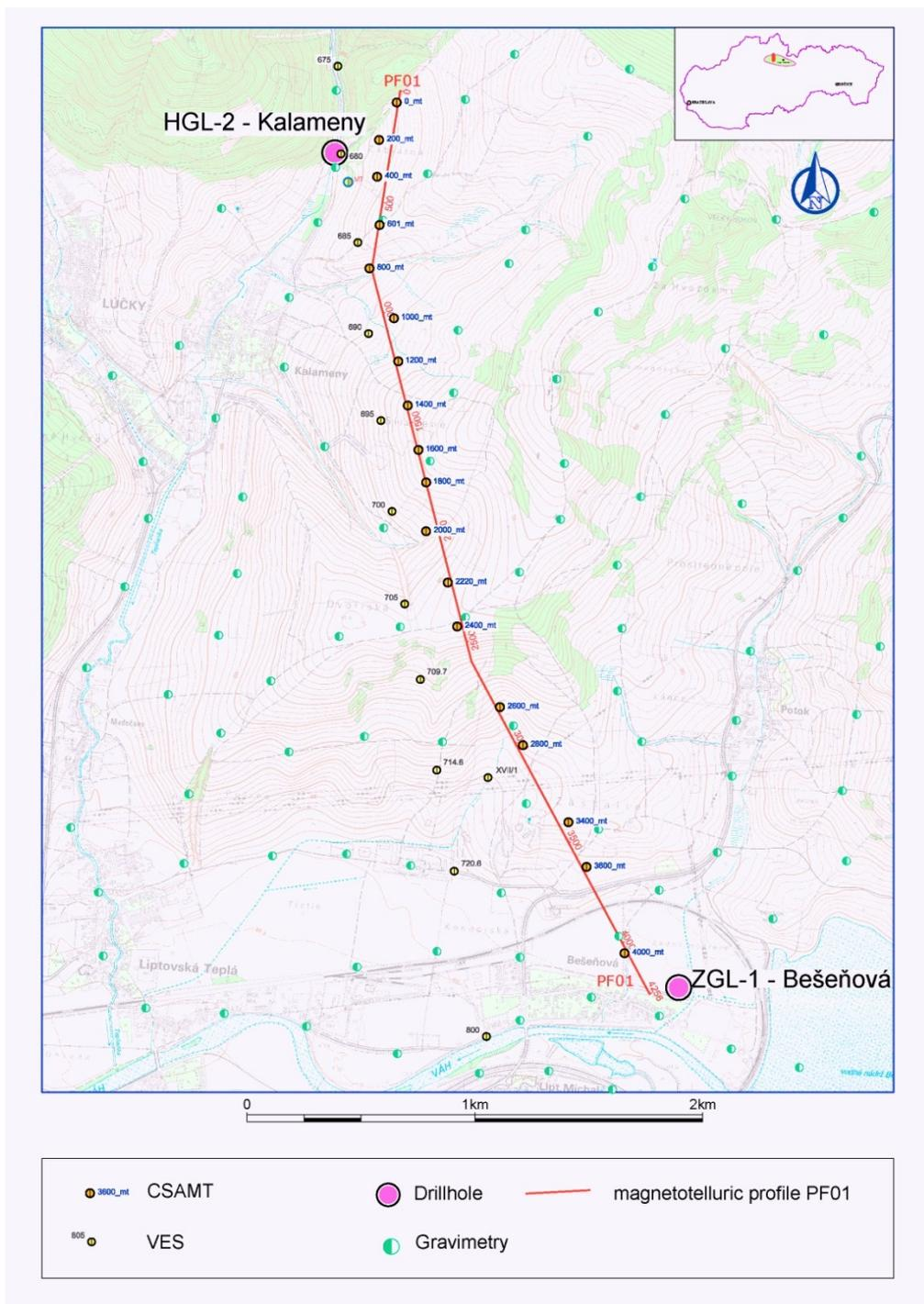
Figure 3: Location of CSAMT measured points and wells in Kalameny and Besenova
