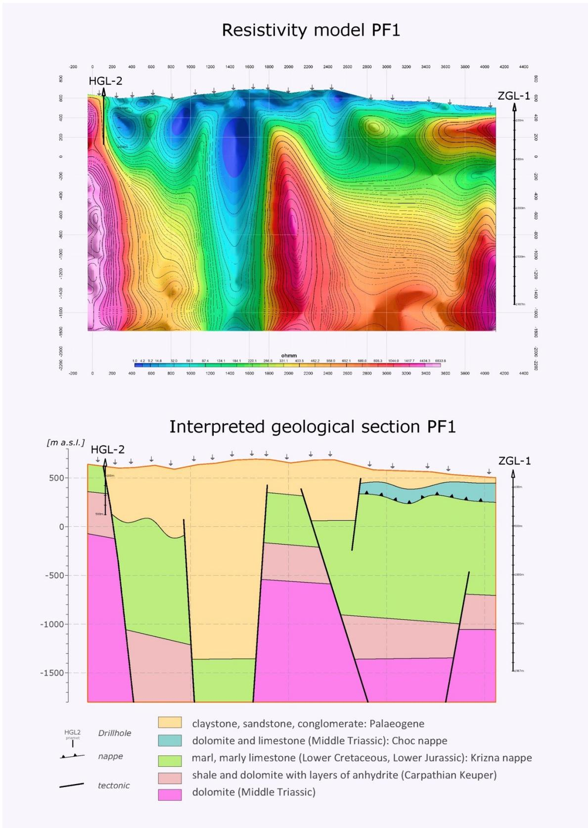
**Figure 6: Geophysical isohohmic profile and its geological interpretation**
